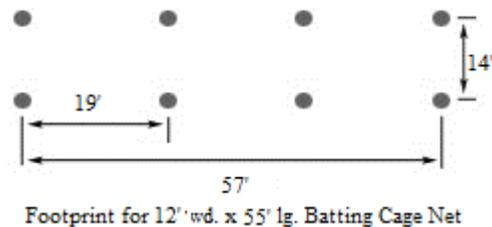
The frame is designed to be 57' long by 16' wide with a 14' wd. net and 57' long by 14' wide with a 12' wd. Net. The Footprint of the frame is 2' wider and longer than the footprint of the net. This will allow the net to slow a ball more before it hits the frame, thus reducing the speed of ricochets.
