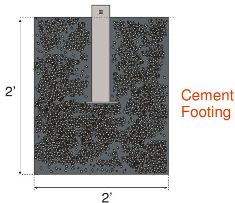
\*This illustration shows the bolt hole exposed, however some customers elect to mount the sleeve flush with the ground to avoid hitting the sleeve with lawn maintenance equipment.\*\*.
