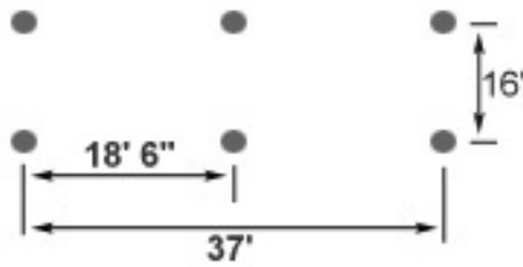
The frame is designed to be approximately 37' long by 16' wide, which is larger than the footprint of the net itself. This will allow the net to slow a ball more before it hits the frame, thus reducing the speed of ricochets.
